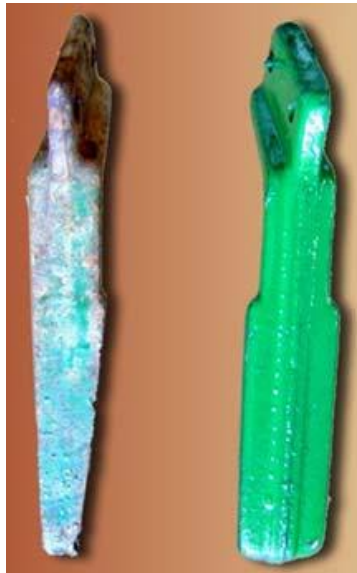
Bullseye Tube with additional wear allowances (left) Standard Tube (right).
